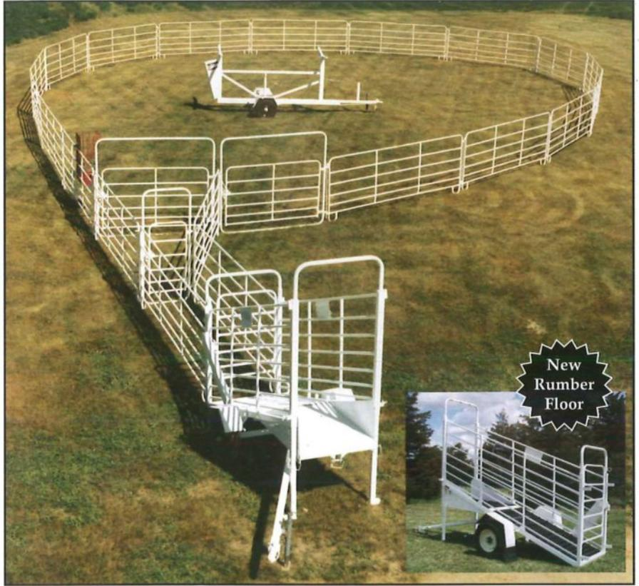
Entire corral loads easily into 12' x 38" chute for easy transportation. Chute adjusts from 26 inches to 52 inches in height for ease in loading or unloading at any level. This chute is equipped with torsion axle, radial tires, fenders, mud flaps, tongue that swings sideways out of way, jack, built in rear gate, and extension hangers to allow a dozen extra panels or a working alley to be hauled. All stationary and portable chutes have the new Rumber flooring.
